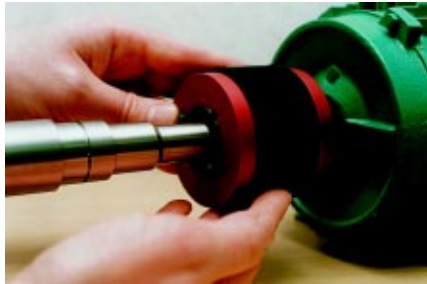
Insert screws and locate on shaft.
