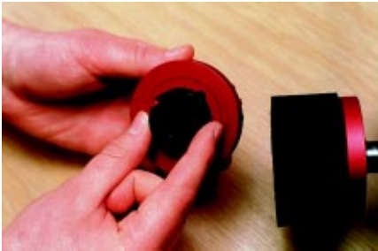
Insert bush into end piece.
